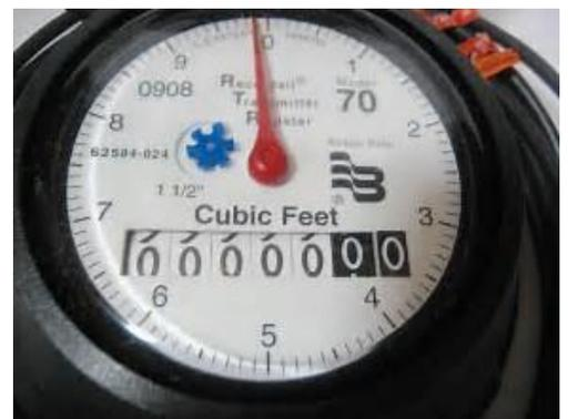
If the needle has moved or the numbers have changed, you have a leak (probably a slow one. If you have a larger leak, you will see the needle moving right away.) One rotation of the red dial is about 7.5 gallons.
