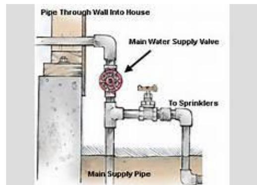
Turn the supply valve to the off position. (Be careful to turn the valve slowly, older valves can break easily.) Run a faucet inside your home to verify that the flow of water stops completely. Go out to the water meter and see if the rotation stops. If it stops, the leak is on the house side of the supply valve. If the rotation does not stop, the leak could be on the water pipe running between the water meter and the water supply valve.
